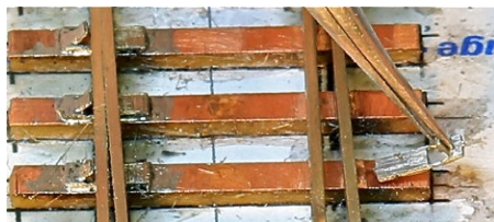
Figure 7. A slide chair is held by its claw and slid between rail and sleeper from the side...
