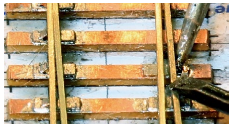
Figure 10. ...trapped in position by pressing down on the rail and soldered...
