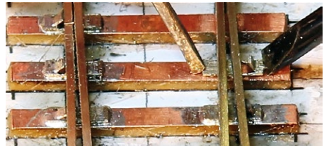
Figure 9. The slide chair is manipulated into position – centred on the sleeper and square-on to the rail...
