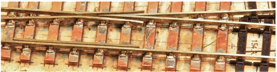
Figure 21. One side of the finished crossing shown in Figure 17, using check and plain chairs. Either side of the check chair used at the knuckle, check chairs have been halved along their half-etched cut lines to make the one-sided chairs needed here. The etched chairs stand up well against the moulded ABS Easitrac sleepers of the plain track on the right. The flangeway below the check rail looks too narrow (it isn’t) because it has been filed down 0.1-0.2mm like the wing rail so that chemical blackening won’t be rubbed off here either when the track is cleaned.
