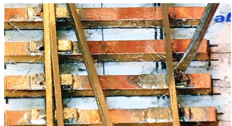
Figure 11. ...and the claw pushed in to match the adjacent chairs.
