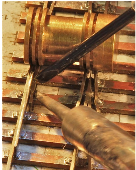
Figure 15. Pushing down obliquely onto the check rail with your prodder (e.g. the small jeweller's screwdriver used here) traps it against the gauges and stock rail and presses it down onto the chair whilst it is soldered.
