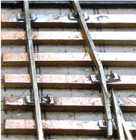
Figure 20. A soldered crossing. Two plain chairs are holding the stock rail and closure rail at the top of the picture. A check chair has been fixed under its stock rail opposite the crossing nose. A check chair is also being used at the knuckle, and where there is no room for an inner claw at the end of the wing rail either a slide or check chair has been made one-sided by trimming at its half-etched cut line. The crossing nose is “chaired” by a sliver of 0.25mm/0.010” shim (scrap etch) on each sleeper. This also nicely demonstrates how the head of the wing rail has been filed down (0.1-0.2mm) at an angle so that metal blacking (or painting) will not be rubbed off when the track is cleaned, and only the true running surfaces of the rail head will stay shiny. Fabrication of the jig to achieve this is described in the Association’s book “Track”.
